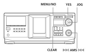
Turn the JOG dial until the disc number to which you want to assign a Disc Name appears in the display.
